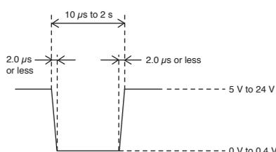
Voltage reading shows figure by terminal with 10 kΩ or more.
